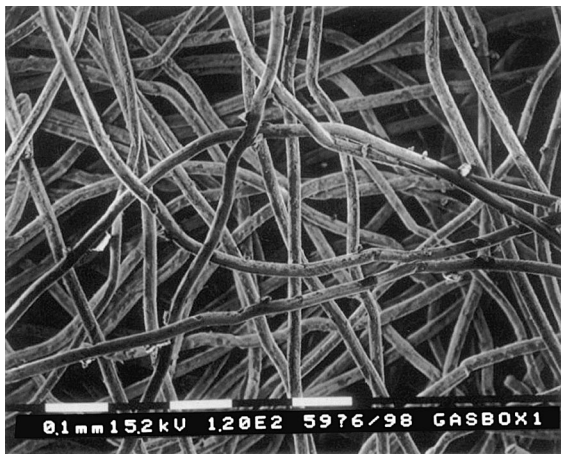
Fig. 2. SEM microstructure of a felt tile. The felt parameters are: d = 25 \mu\text{m} , V_f = 15\% and t = 13 \text{ mm} .
